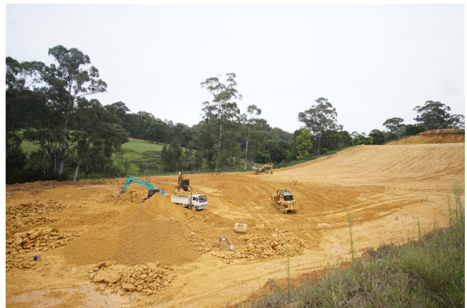
Figure 11. Contractors at a quarry in the Gippsland region loading limestone rock for reef construction, Victoria, 2022. © Scott Breschkin
